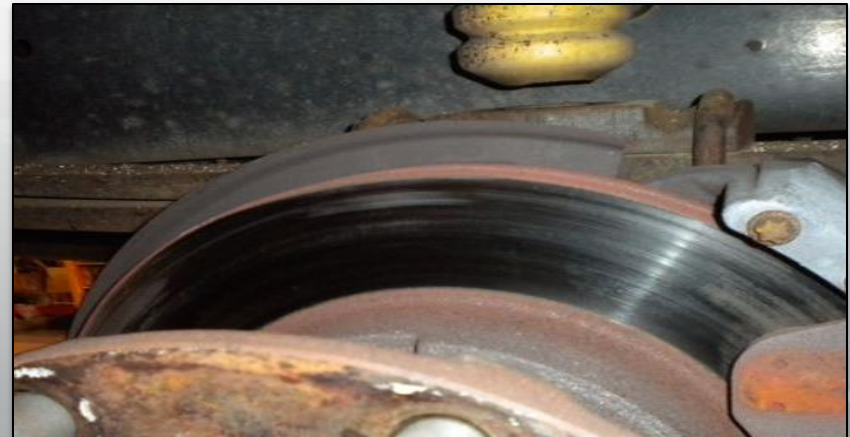
Light pad transfer on face of rotor-Normal Condition-no replacement needed
